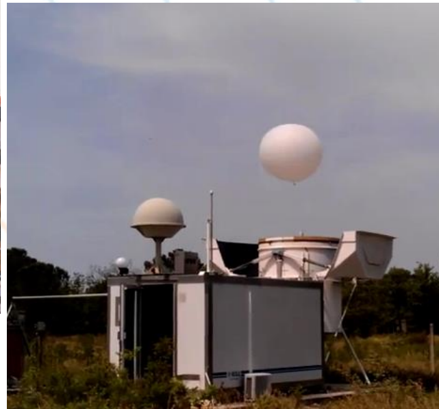
Radio-sounding system in Zagreb and Zadar (modernized in 2017 to new RS-41 Vaisala automatic system)
